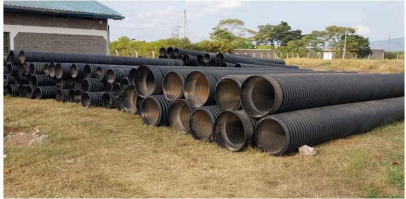
HDPE Sewer pipes
